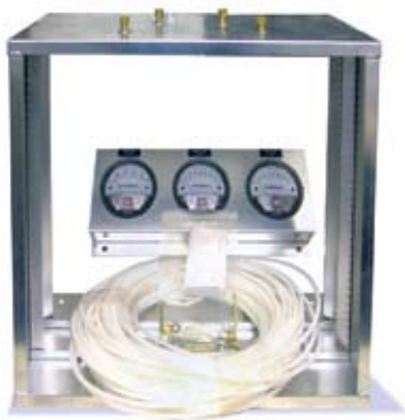
Figure 3: 3-Stage Monitoring System, magnetic gauges monitor the pressure differentials across each filter stage.
