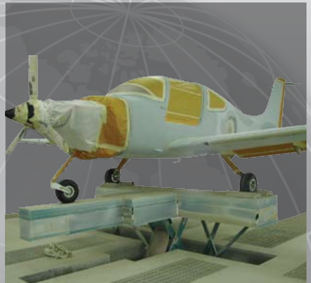
Painting small planes with a lift designed to allow for the dropping of the aircraft so part of it is below grade makes it easier for the painter to paint the top parts of the fuselage and maybe even the empennage.
