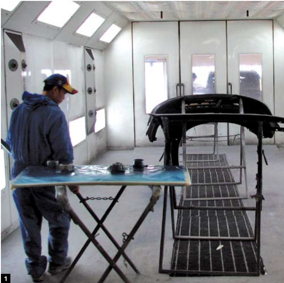
1. Good practice—the floors are clean, there is nothing in the corners, and the parts racks are placed directly over pit.
